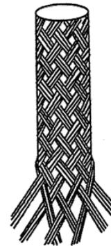
Fig. 3. Flat braided fabric structure (Adanur et al., 2003).
