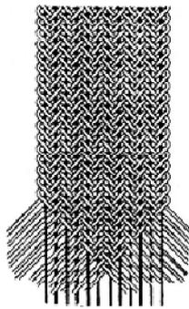
**Flat braids:** Flat braid is made in the form of tape or flat strip. Tubular braiding machine have even number of carrier but flat braids have odd number of carriers. Size of the braid fabric is decided by number of carriers, linear density of yarn and number of yarns per carrier. Figure 3 shows the flat braided fabric structure (Adanur *et al.*, 2003).
