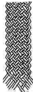
Fig. 4. Triaxial braided structure (Adanur *et al.*, 2003).
