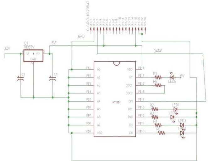
Fig. 3. Schematic of transmitter module.
