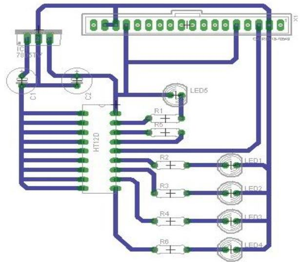
Fig. 4. PCB layout of transmitter module.
