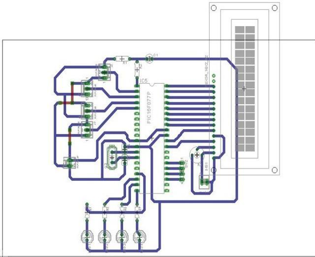
Fig. 5. Schematic diagram of receiver module.
