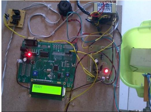
Fig. 9. Sensor triggered and dustbin full status.
