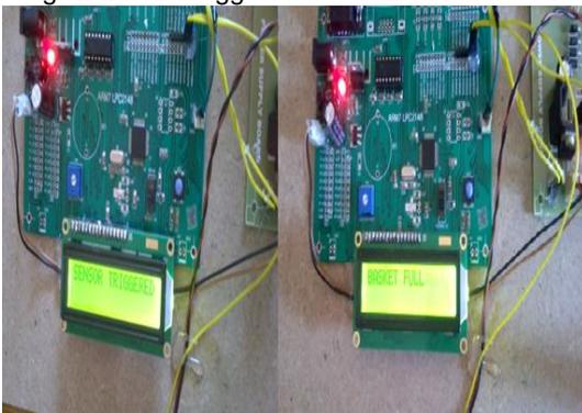
Fig. 10. Waste collecting robot status.
