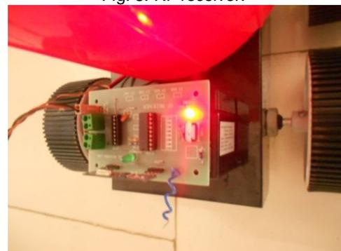
**Encoder (HT12E):** The encoder will convert 8 address bits + 4 data bits into serial form for transmission. The transmitter enable pin is pulled low. Upon receipt, transmitter enable the HT12E begins a 4-word transmission cycle and this cycle repeats until the transmitter enable pin pulled low.
