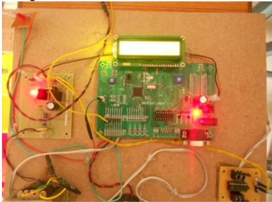
**Decoder (HT 12D):** The serial address and data received by RF receiver is converted into parallel using HT12d decoder. This conversion depends on the no error status. The conversion causes to pull a high signal at valid transmission (VT) pin of the decoder.
