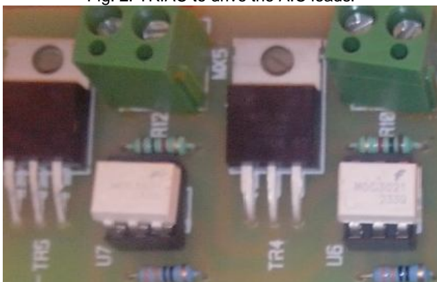
Fig. 2. TRIAC to drive the A.C loads.
