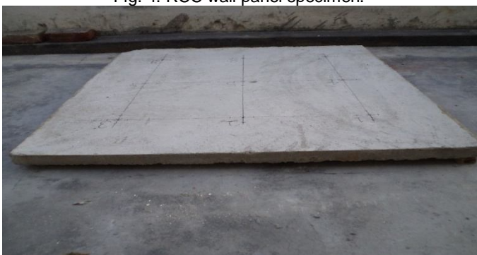
Fig. 4. RCC wall panel specimen.
