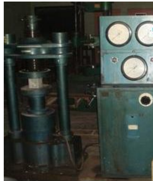
Fig. 1. Test set up for compressive strength test of concrete.
